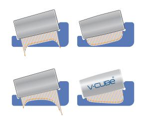
Accurate line contact between the rollers and raceways ensures optimum stress distribution at the contact points and prevents stress increases at the edges. As a result, the bearings can tolerate certain angular misalignments and give better support to moment loads.
